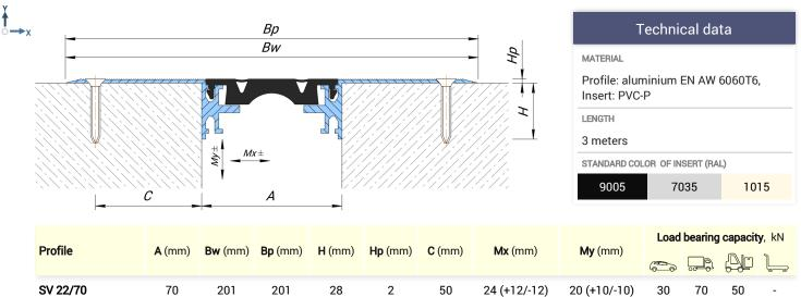
$\hbox{!} \ \hbox{With heavy traffic, the flexible insert will be subject to wear.}$
