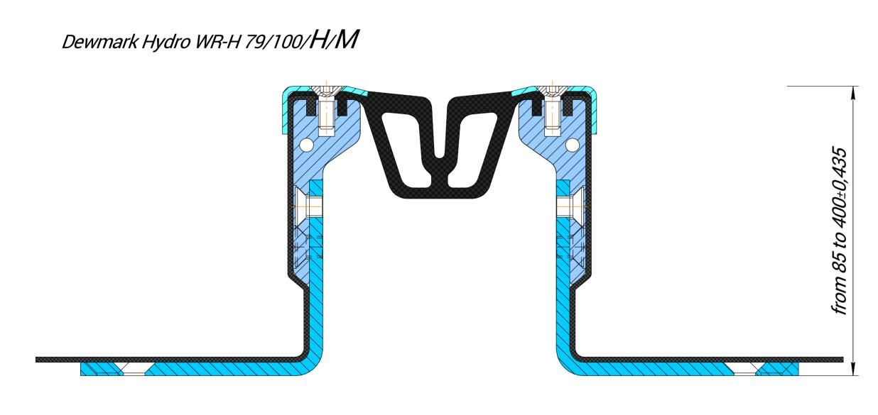
The profile is made to a specific height H from 85 mm to 400 mm.
