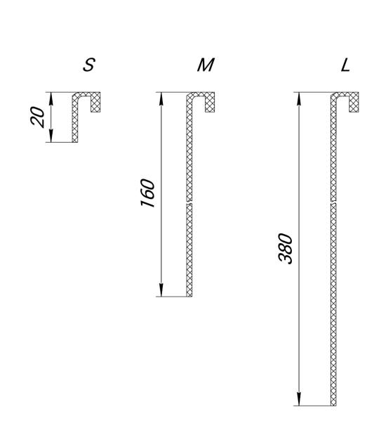
A profile can be completed with three types of sheets: S - small - 20 mm wide, M - medium - 160 mm wide,
