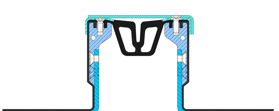
The profile is made to a specific height H from 85 mm to 400 mm.
