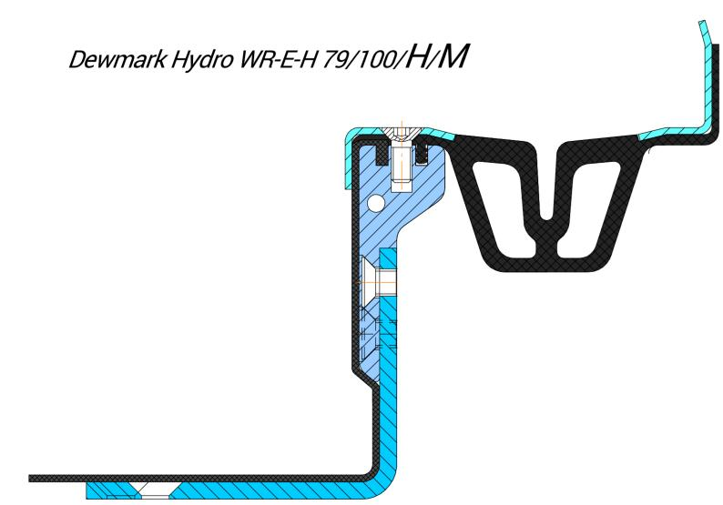
The profile is made to a specific height H from 85 mm to 400 mm.
