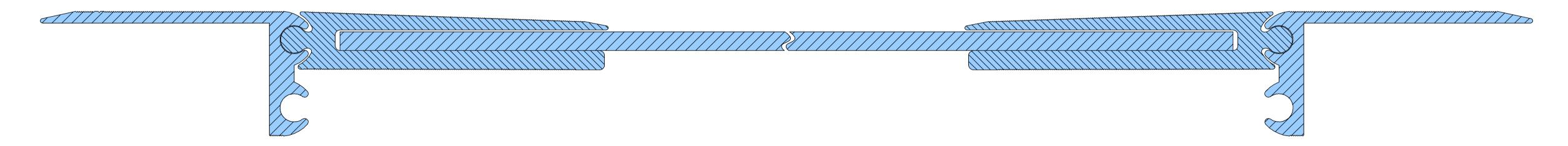
The profile is made for a specific width of the expansion joint "A" (mm) from 300 to 1000 mm
